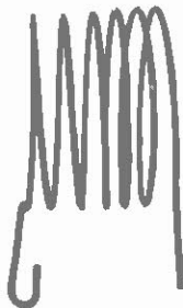
1st speed resistor 6 gauge with 5 turns
