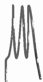
3rd speed resistor 7 gauge with 3 turns
