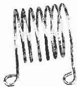
First speed resistor. Nine gauge wire
