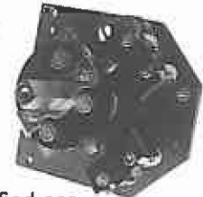
Beefed up F&R switch for modified car. If a high amp controller is installed you need this switch
