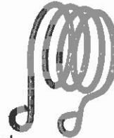
Third speed resistor. Six gauge wire
